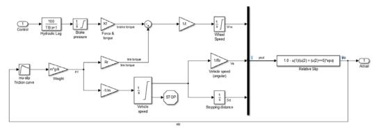
The Brake System Dynamics subsystem is complex. What follows is a high-level examination of how it works. For a more detailed analysis of a similar system, see Modeling an Anti-Lock Braking System.
